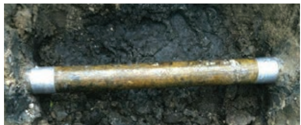
Superficial oxidation of cast iron pipe since 1958
