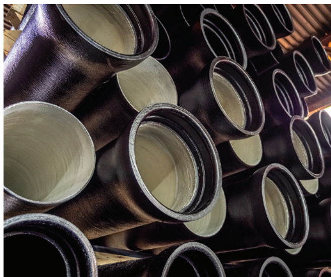
Ductile iron pipe without a seal-coat lies ready for shipment. Eliminating the seal-coat is now an option for manufacturers unless otherwise specified.
